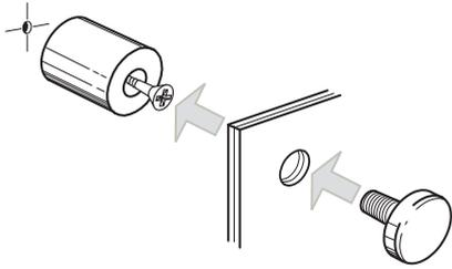
**Two Part Fitting** - Includes M10 Stud-Cap and Standoff Spacer/Barrel.
